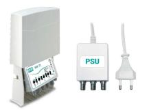
1-input (III+DAB+UHF) mast amplifier with 42dB gain and up to 116dBµV output level on UHF band, separate VHF/UHF amplification with independent gain adjustment (0-15dB) for each band and low noise figure. T2 technology with UHF cut band for LTE 4G @790MHz and 5G @694MHz. **Power supply included in the package.**
